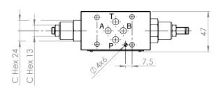
All stackable valves AM3-FC-\* conform with ISO and CETOP specifications for mounting surface dimensions. Valves height 40 mm. Leakage between valve and mounting surface is prevented by the positive compression on their seats of 4 seals of OR type. All valves have on their "mounting" surface a ø 4 mm cylindrical hole and have on their "seals" surface a ø 3 mm cylindrical hole, conform with ISO and CETOP norms.
